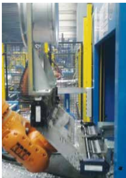
GRR Grippers shown without guards which protect the guide shaft from machine chips
